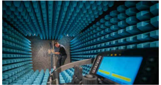
Verification Engineer prepares for radio frequency tests in one of Scanreco's laboratories and EMC chambers.
